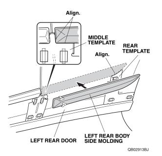
17. Press on the left rear body side molding firmly with the palm of your hand while removing about 50 to 100 mm (2.0 to 4.0 in.) of the adhesive backings at a time.
