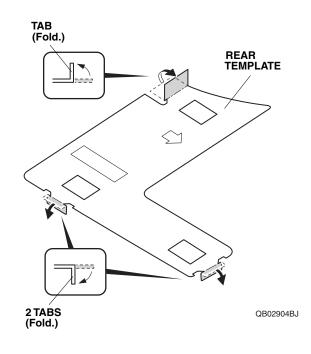
8. Align the two tabs of the rear template onto the edge of the left rear door as shown.
