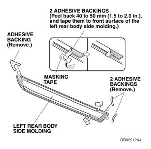
16. Align the left rear body side molding with the middle and rear templates, and install the left rear body side molding on the left rear door.
