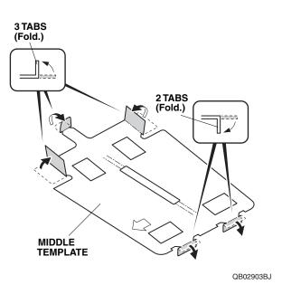
5. Align the middle template onto the left front and rear doors as shown.
