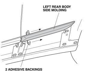
(Press on the left rear body side molding firmly with the palm of your hand while removing the adhesive backings.)
